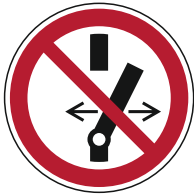
P031 Do not alter the state of the switch
