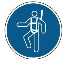
M018 Wear safety harness
