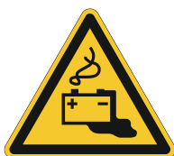
W026 Warning; Battery charging
