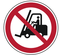
P006 No access for fork lift trucks and other industrial vehicles
