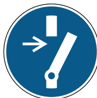
M021 Disconnect before carrying out maintenance or repair
