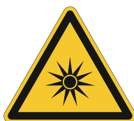
W027 Warning; Optical radiation
