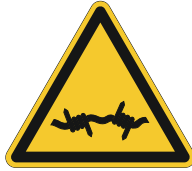
W033 Warning; Barbed wire
