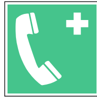
E004 Emergency telephone
