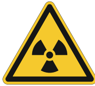
W003 Warning; Radioactive material or ionizing radiation
