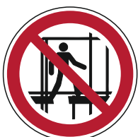
E025 Do not use this incomplete scaffold
