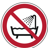
E026 Do not use this device in a bathtub, shower or water-filled reservoir
