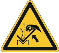
W031 Warning; Hand crushing between press brake tool
