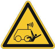
W037 Warning; Run over by remote operator controlled machine
